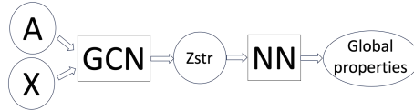
Fig. 2. Regression model based on a GNN. Input: Node features X and adjacency matrix A . Z_{str} is the latent domain.
