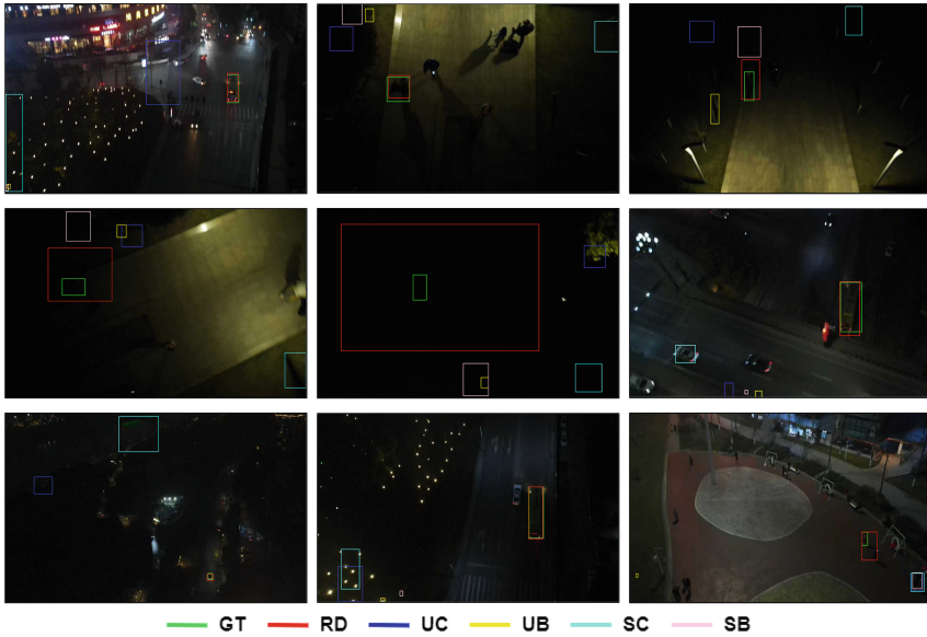
Fig. 5. Visual comparison of results of RADA and baselines on the test set of NAT2021-L dataset. Here, GT is ground truth, RD is RADA, UC is UDAT-CAR, UB is UDAT-BAN, SC is SiamCAR, and SB is SiamBAN.
