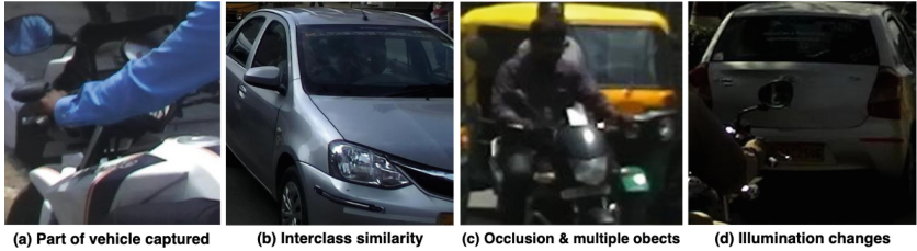
Fig. 5. Illustration of challenges in FGVD dataset: (a) part of the vehicle captured; only a part gets captured due to moving traffic, (b) interclass similarity; many cars appear highly similar and are difficult to identify from the front view, (c) occlusion and multiple objects; the autorickshaw is occluded by a motorcycle, and (d) illumination changes; due to changes in daylight & weather conditions.
