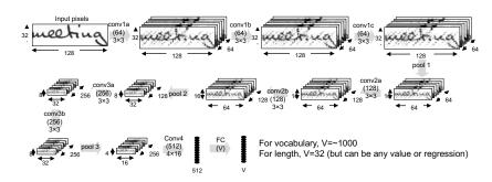
$C(64,3,3)-C(64,3,3)-C(64,3,3)-P(2)-C(128,3,3)-C(128,3,3)-C(256,3,3)-P(2)-C(256,3,3)-C(512,3,3)-C(512,3,3)-P(2)-C(256,4,16)-FC(V)-SoftMax\ where \\ C(D,H,W)\ stands\ for\ convolution\ with\ the\ dimensions\ of\ the\ filter\ as\ HXW\ and\ the\ depth\ D.\ Each\ convolutional\ layer\ is\ followed\ by\ a\ batch\ norm\ and\ ReLU\ layer.\ P(2)\ represents\ a\ 2\ X\ 2\ pooling\ layer\ with\ stride\ 2.$
