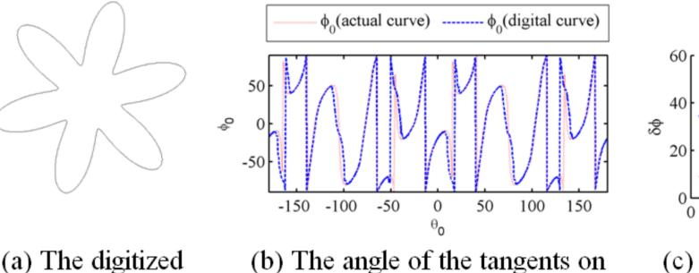
(b) The angle of the tangents on the actual curve and the digital represented by (22) curve (using R=20)
