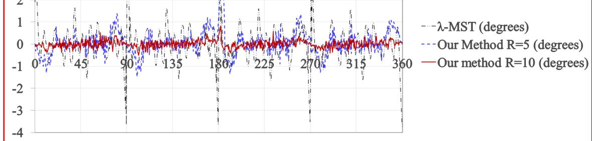
Average absolute error in the computation of tangents for 100 experiments with digitized circles of radius 100 and centers within 1 pixel region chosen randomly. The result is compared with  $\lambda - MST$  estimator.
