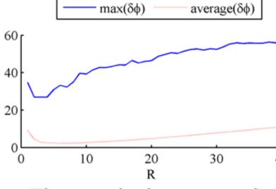
(c) The error in the computation of the tangent due to digitization for various values of R
